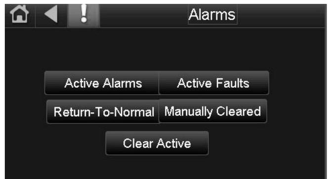
The alarm must be reset in the program by turning the selector switch from the ON to the OFF position. Wait for the exclamation point to turn gray before turning the controller back on. This alarm clearing process may take 5-10 seconds to update. The alarm will reoccur if the fault has not been corrected.
